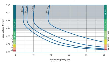
Natural frequency of a single-degree-offreedom system consisting of a fixed mass and an elastic bearing consisting of VIKAFOAM VF 110 on a stiff subgrade.
